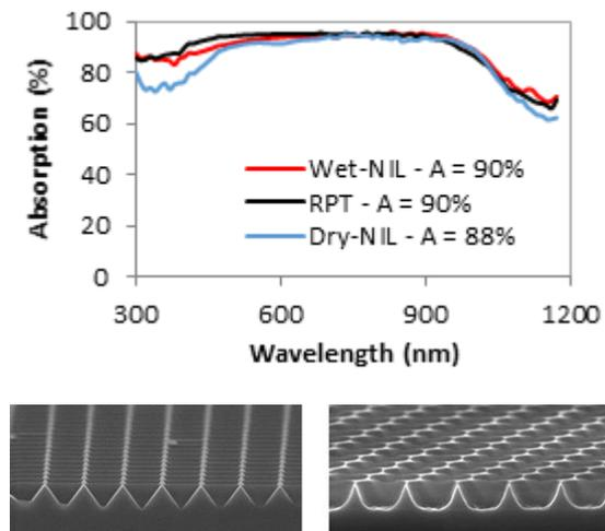
**Figure 3:** Optical absorption as measured on IBC cells on  $40\mu\text{m}$  silicon foils. Curves are shown for random pyramid texturing and NIL based texturing. The wet-etched and dry-etched NIL textures are shown in the tilted SEM photographs below (the pattern has a period of  $800\text{nm}$ ).
