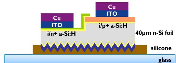
**Figure 1:** Schematic cross-section of the heterojunction IBC cell on bonded silicon foils.
