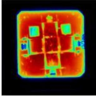
**Figure 6:** Photoluminescence (PL) image of a bonded n-type FZ substrate after emitter patterning and re-passivation with a-Si:H (i/n<sup>+</sup>). The areas with lower PL intensity correspond to regions where a-Si:H (i/p<sup>+</sup>) was etched away, resulting in high surface roughness and less effective passivation.
