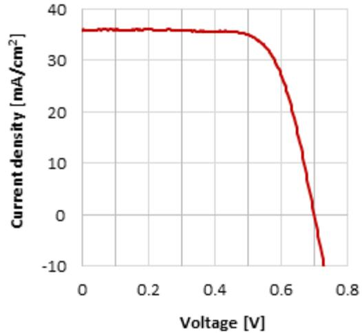
**Figure 4:** Light J-V curve of the best HIT-IBC cell, achieved on a non-textured 200μm n-type FZ wafer. Cell area is 3.96 cm<sup>2</sup>.
