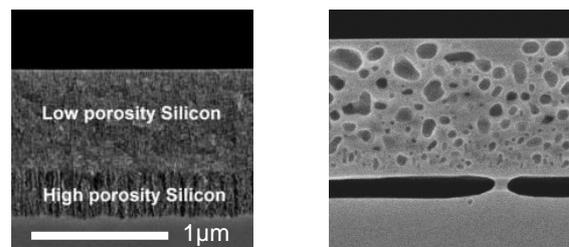
**Figure 2:** Formation of thin silicon foils using porous silicon etching (left-hand image) followed by high temperature anneal in hydrogen (right-hand image). The resulting restructured porous-Si layer serves as a template for subsequent epitaxial deposition.
