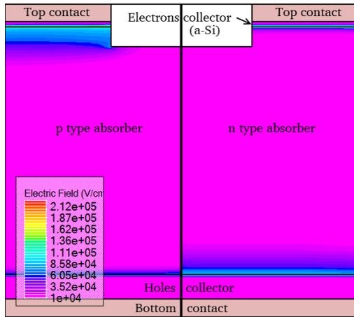
**Figure 9:** Map of the electrical field at maximum efficiency for a variation of the structure presented in figure 4 where the pattern would be fabricated after a-Si deposit (ITO has been replaced by a metal electrode).
