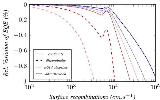
**Figure 6:** EQE variation (light colors stand for a p type absorber and dark curves correspond to a n type absorber)
