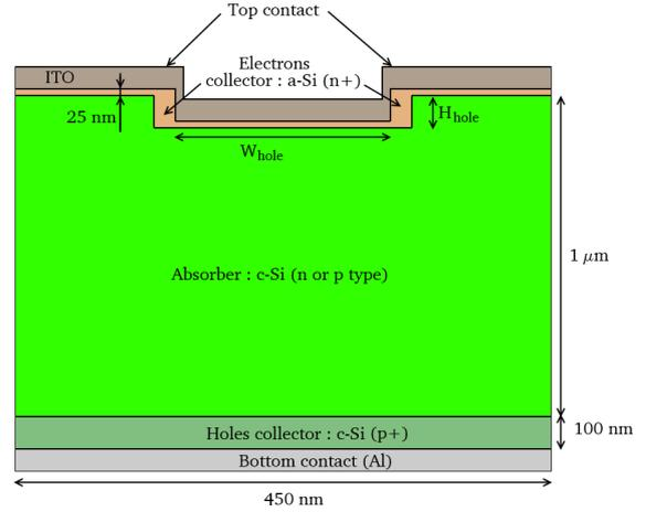
**Figure 4:** Slice view of the device (would correspond to the profiles in fig 2, with no through holes)
