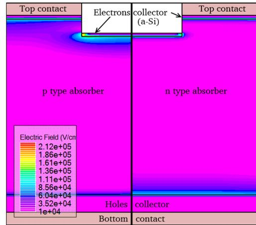
**Figure 7:** Map of the electrical field at maximum efficiency for a variation of the structure presented in figure 4 where no a-Si covers the sidewalls of the patterns (ITO has been replaced by a metal electrode).
