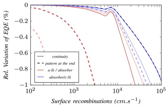
**Figure 8:** EQE variation (light colors stand for a p type absorber and dark curves correspond to a n type absorber)
