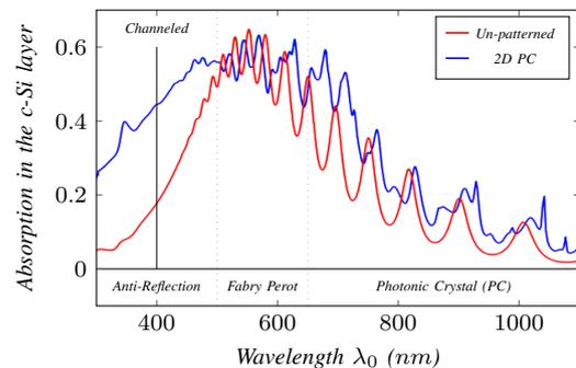
**Figure 1:** Influence of a 2D PC patterning on the absorption spectrum for a thin c-Si absorber
