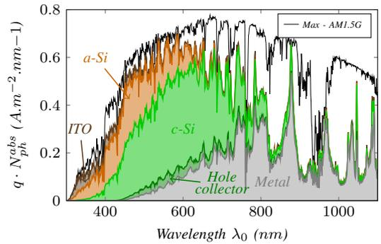
**Figure 5:** Amount of absorbed photons in each part of the device for the optimized design (3D-FDTD)
