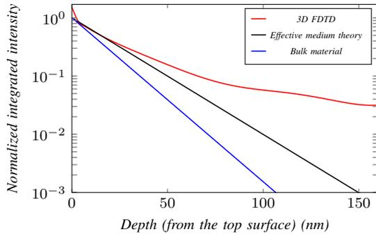
**Figure 3:** Absorption of a channeled signal
