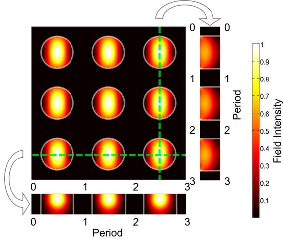
**Figure 2:** Top view of the electric field in a channeled regime into a thin membrane for a spatial period around  $500 \text{ nm}$ .
