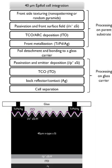
**Figure 1.** Epifoil double side contacted solar cell fabrication process flow sequence (up) and schematic cross section of the final stack (down).
