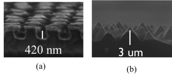
**Figure 2.** Topography of (a) *Dry-NIL* and (b) the reference random pyramid texturing.
