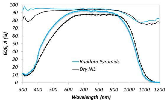
**Figure 3.** Absorption (solid lines) and EQE (lines with marker) for the random pyramid textured and *Dry-NIL* 40  $\mu\text{m}$  cells.
